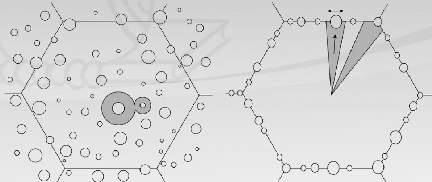
**Figure 1.** Schematic precipitate distributions and diffusion fields (shaded areas) for random precipitation (left) and heterogeneous precipitation at grain boundaries (right) in 2D.
